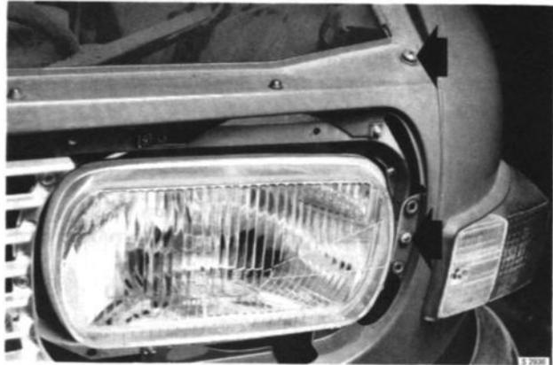
REMOVAL OF FASTENING SCREWS, FRONT PLATE
