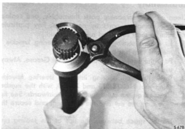
PLACING THE LOCK RING IN TOOL 784161
