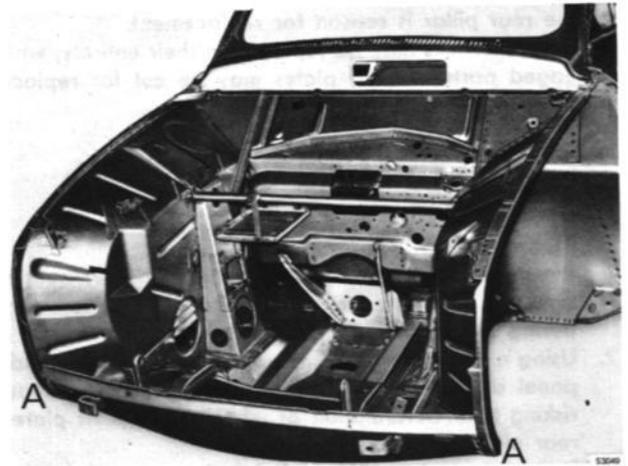
ALIGNMENT OF FRONT CROSS-MEMBER — SECURED WITH BOLTS AT "A".
