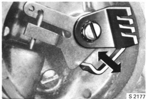
ADJUSTMENT OF THERMOSTATIC SPRING LEVER TONGUE
