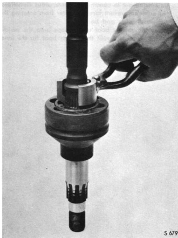
INSTALLATION OF INNER DRIVE SHAFT
