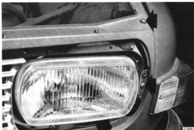
REMOVAL OF FASTENING SCREWS, FRONT PLATE
